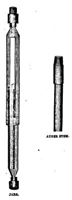
Connected with this auger-stem above is an important arrangement called, technically, "jars," made of two
