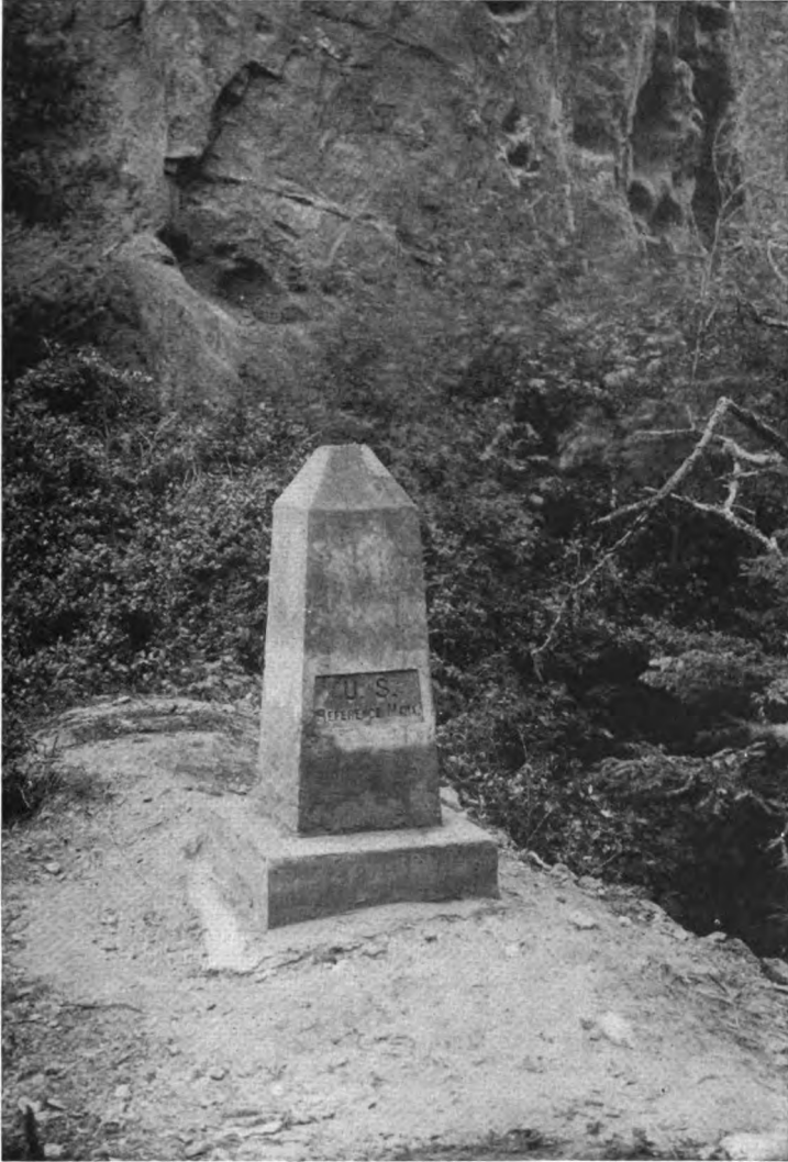
PILLAR POINT REFERENCE MARK, WASHINGTON
